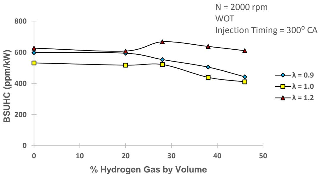
Figure 5: BSUHC against % of Hydrogen Gas at Various Air-Fuel Ratios.
