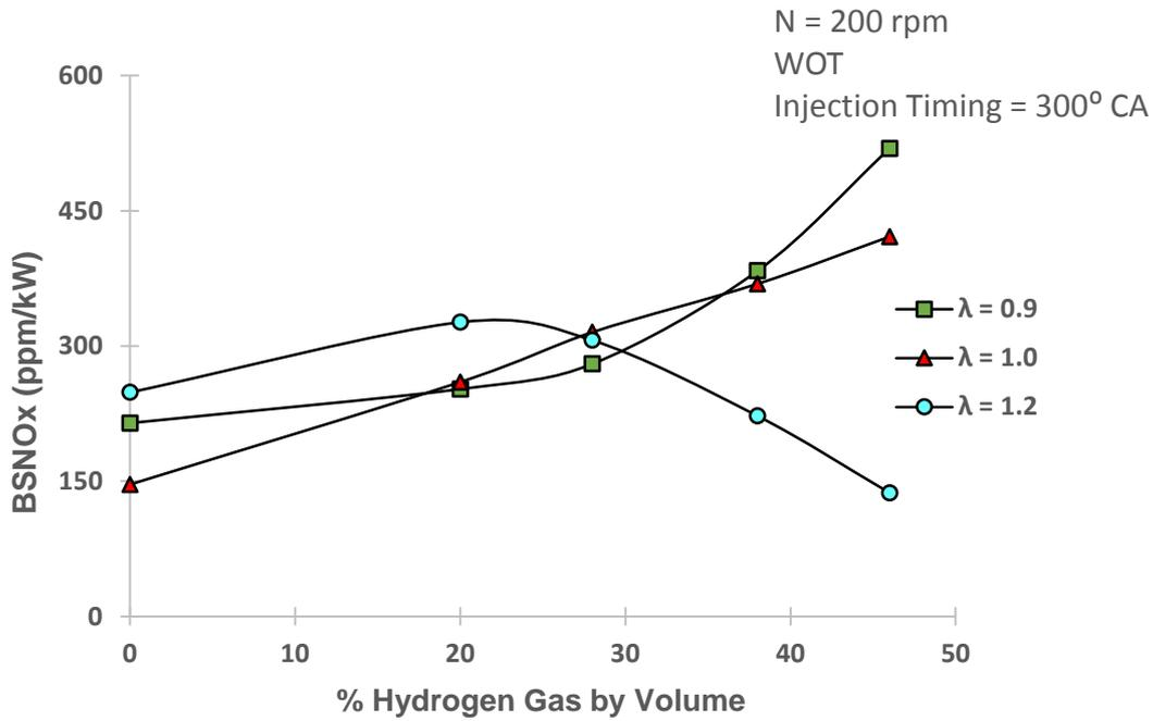
Figure 4: BSNOx against % Hydrogen Gas at Various Air Fuel Ratios.
