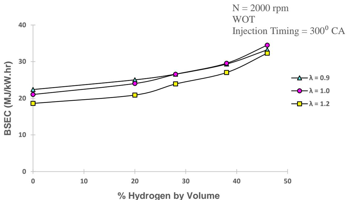
Figure 2: BSEC against % of Hydrogen Gas at Various Air-Fuel Ratios.
