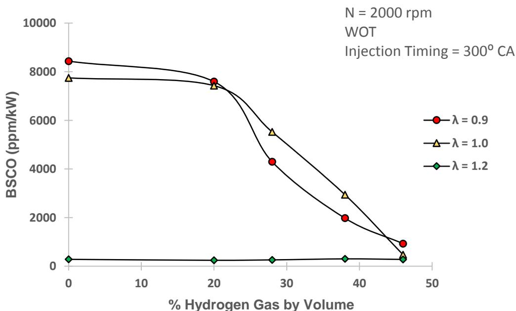
**Figure 3:** BSCO against % of Hydrogen Gas at Various Air-Fuel Ratios.
