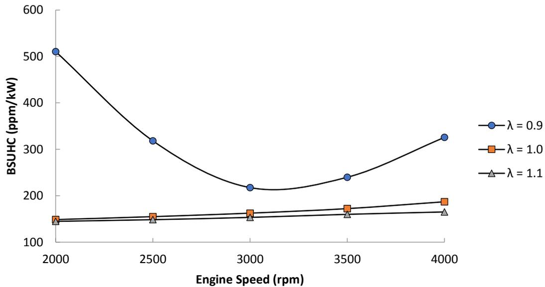
**Figure 6:** BSUHC against Engine Speed at Various Air Fuel Ratios
