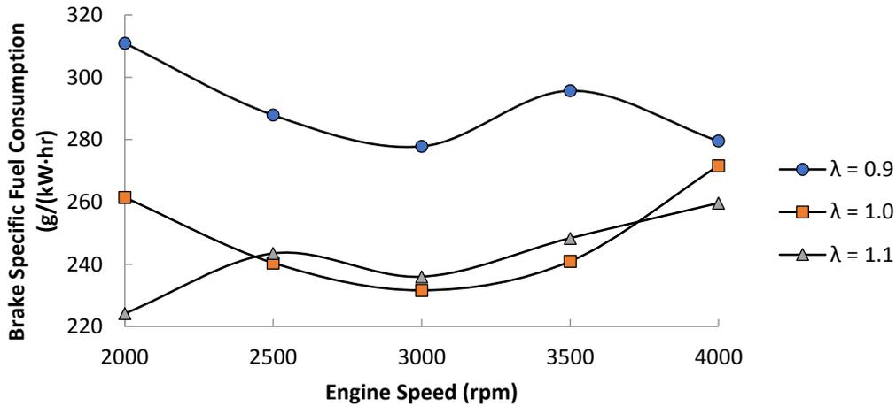
Figure 3: Brake Specific Fuel Consumption against Engine Speed for Various Air-Fuel Ratios
