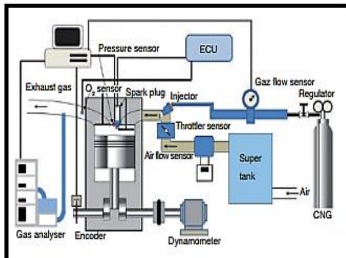
Figure 1: Schematic Diagram of Experimental set up.
