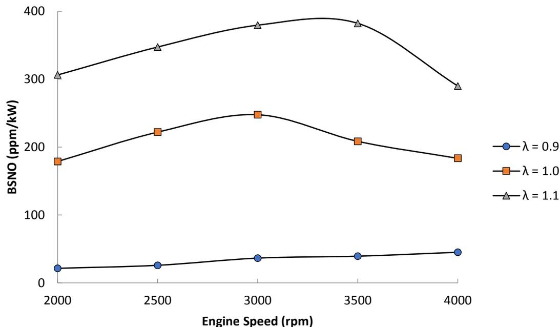
**Figure 4:** BSNO against Engine Speed at Various Air-Fuel Ratios.
