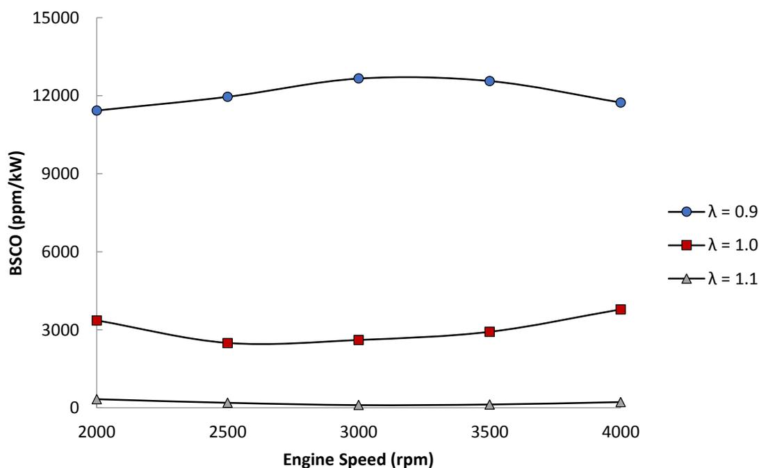
**Figure 5:** BSCO against Engine Speed at Various Air Fuel Ratios.
