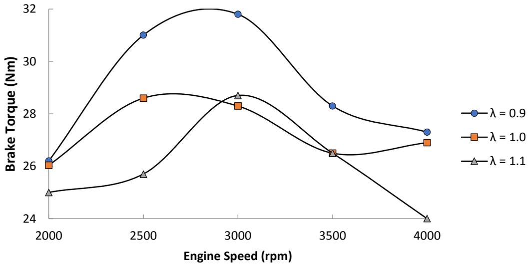
Figure 2: Engine Brake Torque against Engine Speed for Various Air-Fuel Ratios
