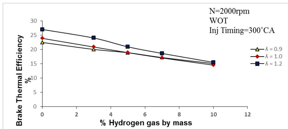
Figure 5: Brake Thermal Efficiency against percentage of Hydrogen at various air-fuel ratios.
