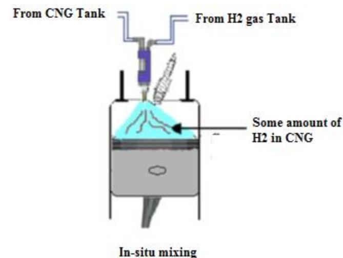
**Figure 2:** In-situ mixing of CNG and Hydrogen gas.
