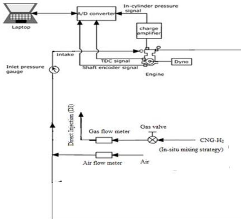
**Figure 1:** Schematic of the experimental set up
