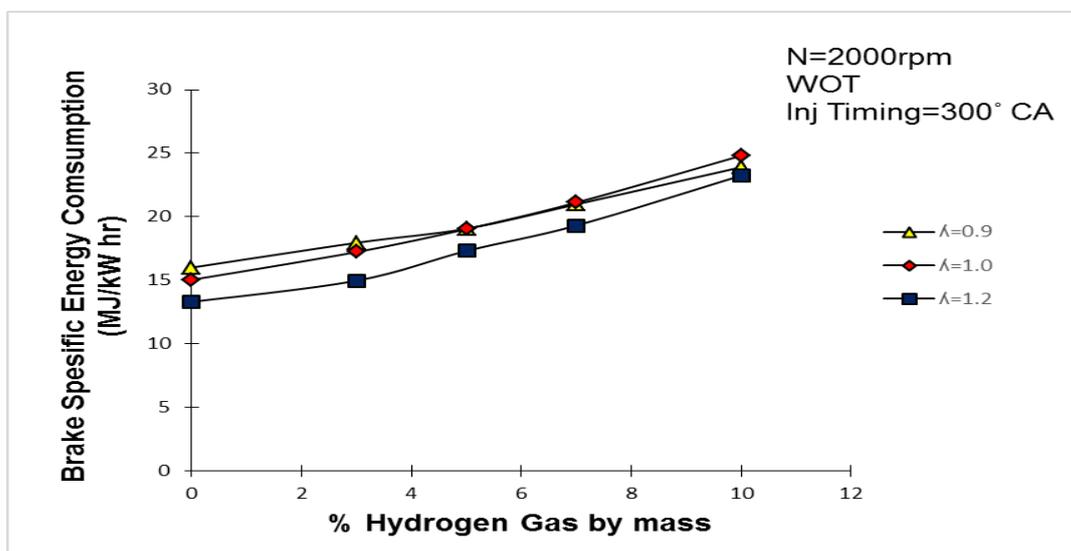
**Figure 4:** Brake Specific Energy Consumption against percentage of Hydrogen at various air-fuel ratios.
