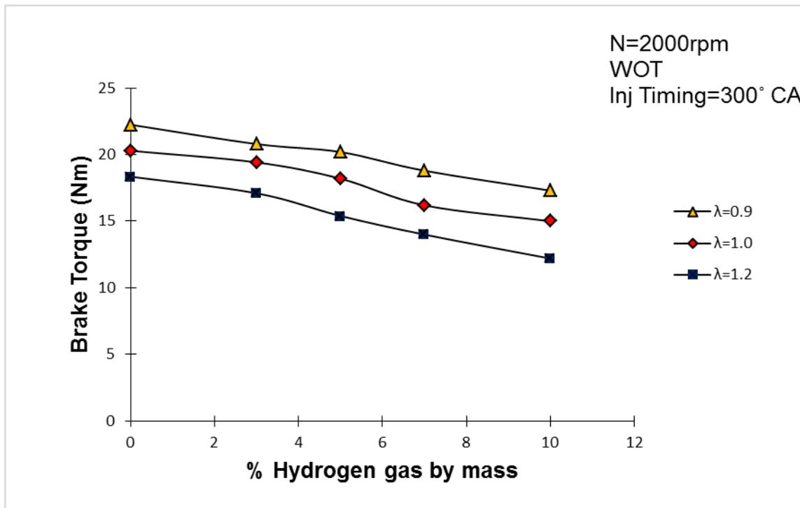
**Figure 3:** Brake Torque against percentage of Hydrogen gas by mass at various air-fuel ratios.
