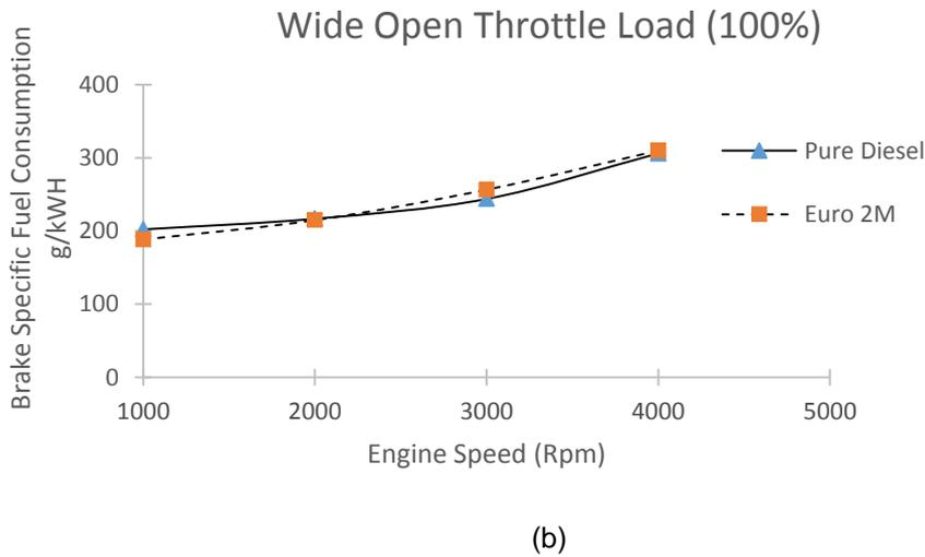
**Figure 4:** Graph of Brake Specific Fuel Consumption vs Engine Speed at (a) idle throttle (20%) load and (b) wide open throttle (100%).
