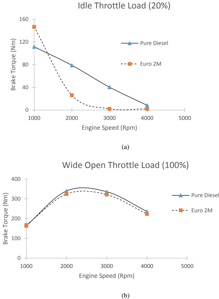
**Figure 3:** Graph of Brake Torque vs Engine Speed at (a) idle throttle (20%) load and (b) wide open throttle (100%).
