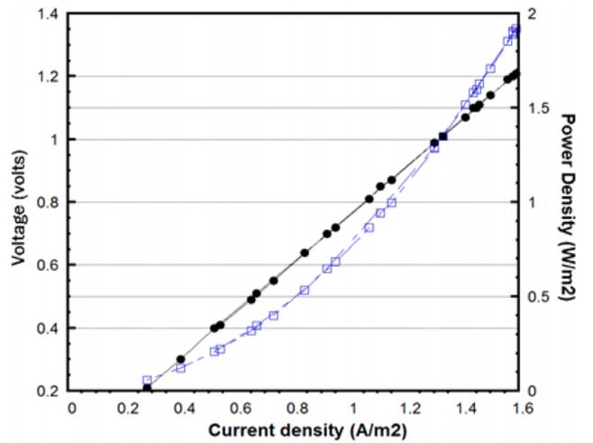
**Figure 6.** Power density, current density against generated voltage in MFC using cow dung seeded with municipal waste water) as substrate
