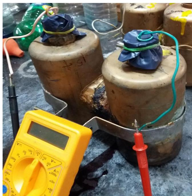
**Figure 1.** Two-chambered Microbial fuel cell set up
