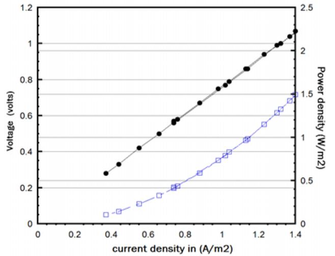
**Figure 5.** Power density, current density against generated voltage in MFC using cow dung as substrate
