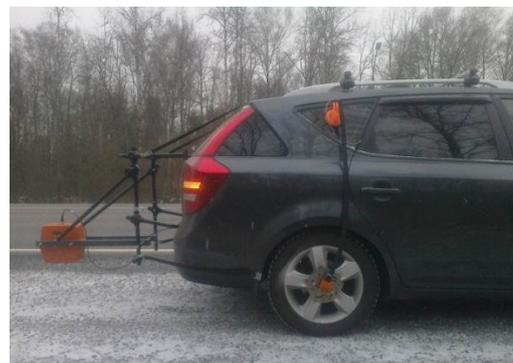
**Figure 5.** Horn antennas block AB -2500R automobile suspension and sensor of passed way.
