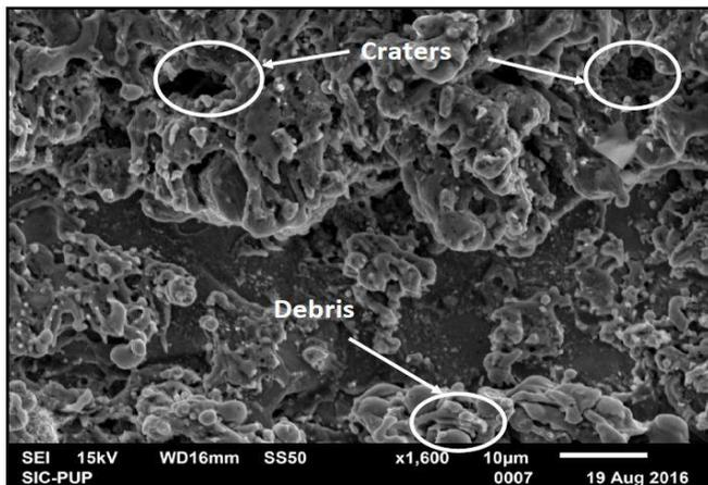
**Figure 8:** Microstructure of machined sample at low level of parameters
