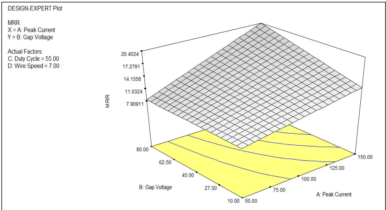
**Figure 3: Peak Current and Gap voltage vs MRR**
