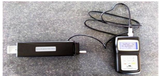
Figure 1 (a) Surface Roughness measuring using Talysurf-surface roughness tester
