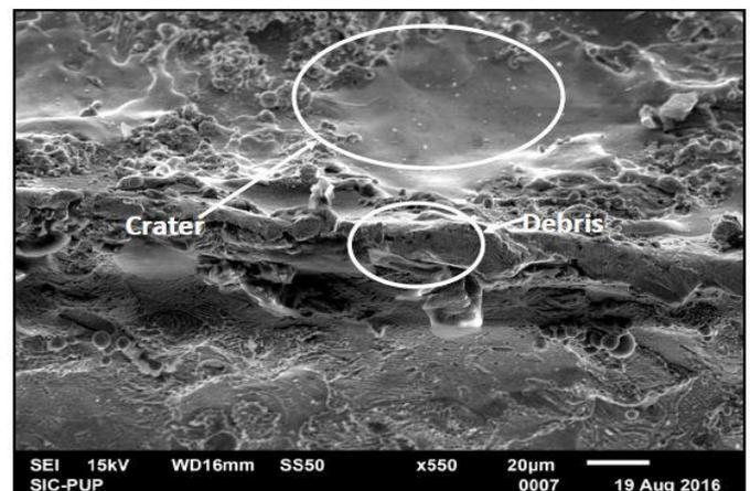
**Figure 7:** Microstructure of machined sample at high level of parameters
