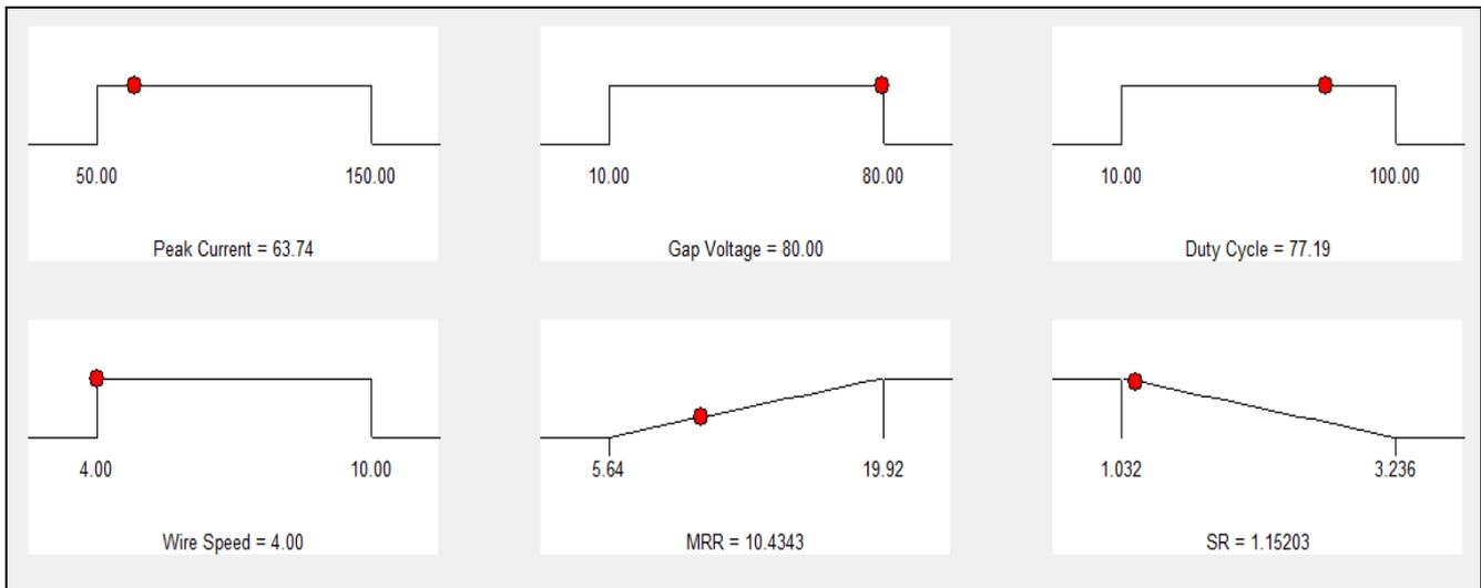
**Figure 6:** Ramp function graph of desirability for multi optimization
