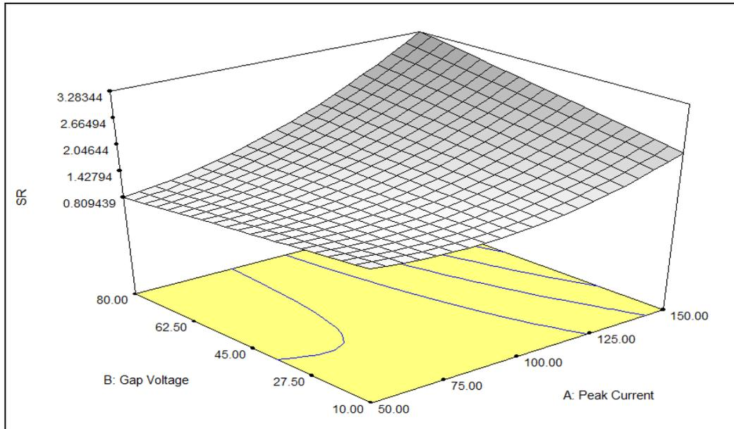
**Figure 4:** Peak Current and Gap voltage vs SR
