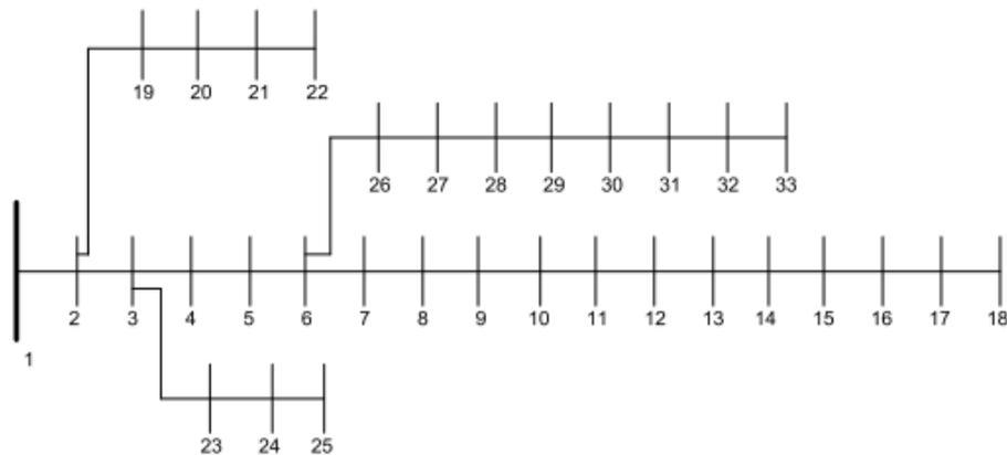
**Figure 4.** System of 33 bars. Source [30]
