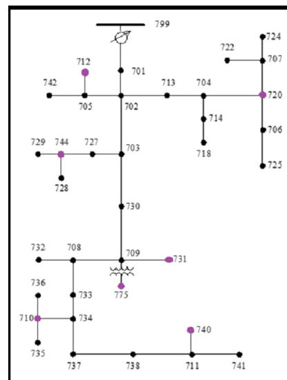
**Figure 4.** Distributed generation nodes in the system.
