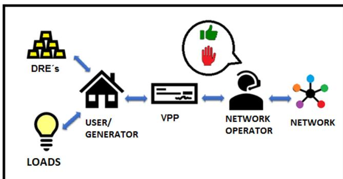
**Figure 2.** Communication of the VPP with agents of the electric market and elements of the electric system.
