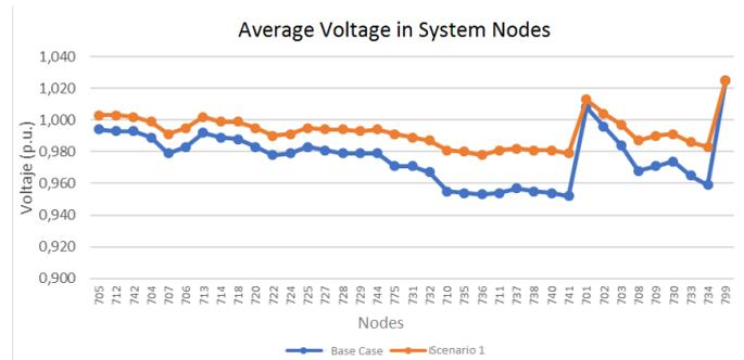
**Figure 5.** Comparison of average voltage profile in system nodes. Basic case study and simulation scenario n° 1 (High demand).
