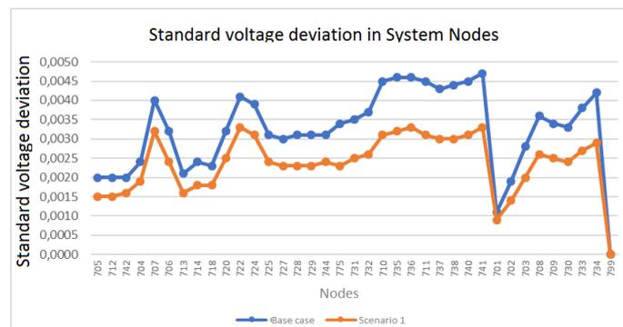
**Figure 6.** Comparison of the standard deviation in system nodes. Basic case study and simulation scenario n° 1 (High demand).
