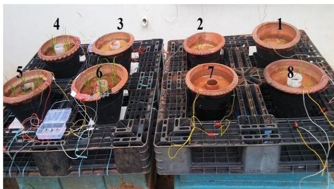
**Figure 2.** Experimental setup of terracotta separator based PMFC
