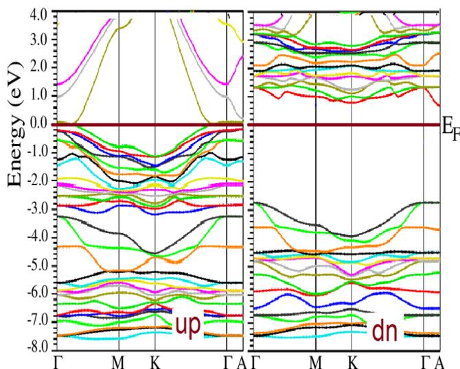
**Figure 3.** Band structure of 1x3-ZnO/MnO multilayer in the wurtzite structure. Source: Authors.
