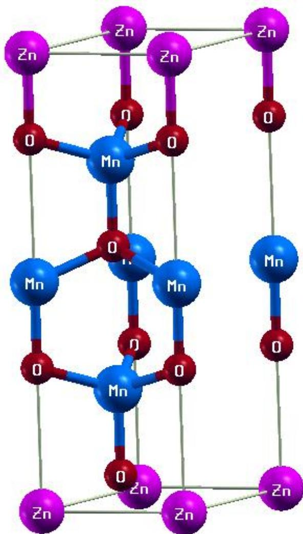
**Figure 1.** Conventional unit cell for 1x3-ZnO/MnO multilayer in wurtzite structure. Source authors
