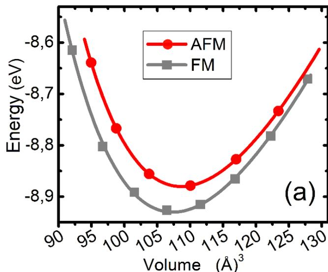
**Figure 2.** Energy vs volume of the 1x3-ZnO/MnO multilayer in the ferromagnetic phase FM (gray color) and antiferromagnetic phase (red color). Data calculated are points and adjusted in the continuous curve. Source authors
