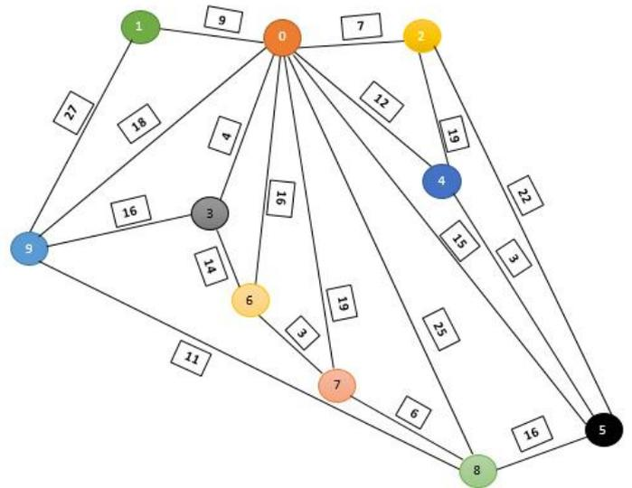
The above Network is the Layout of a city that is being considered for present work, where “0” represents initial point or the Depot and 1 to 9 are the nodes or the delivery points where the orders are to be delivered. The respective distance between the nodes are mentioned in the network diagram. Note: Distance provided is in Km.
