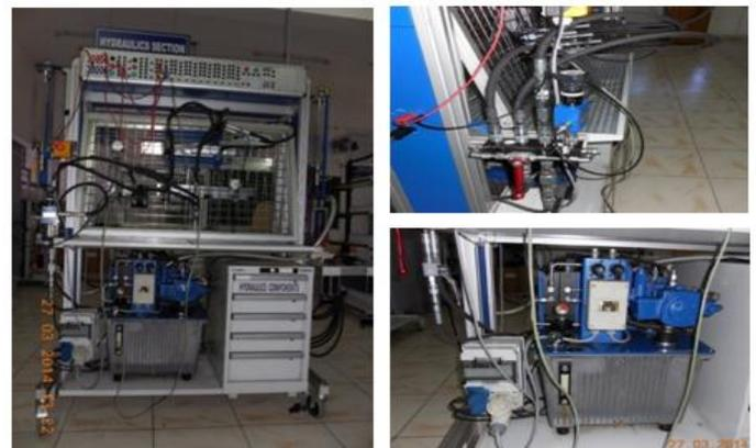
**Figure 4:** Hydraulic system accommodated with hydraulic power pack
