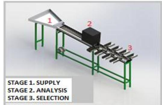
Figure 12. Final Design for classification machine
