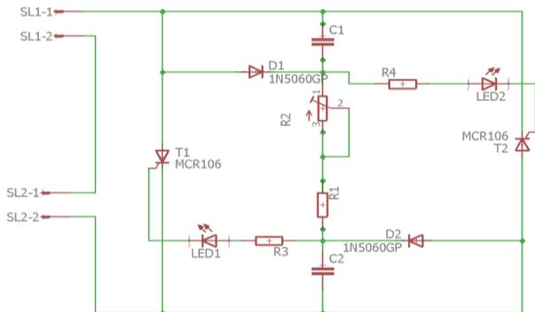
Figure 5. Motor speed control Circuit
