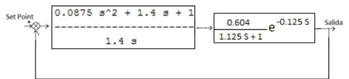
Figure 6. Final block diagram
