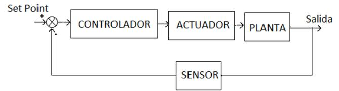
**Figure 2.** Block Diagram to PID Controller
