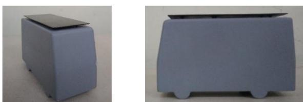
Figure 11. Scaled 3D printed prototype mini bus model with flat solar panel
