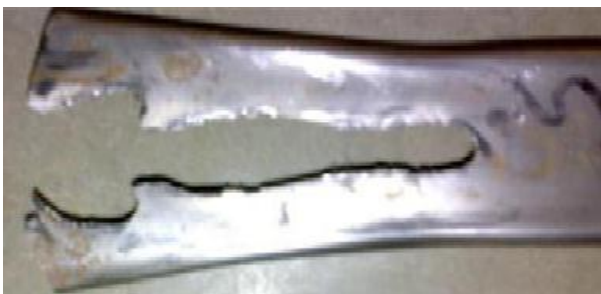
Figure 14: Longitudinal shear failure of 2 mm thick
