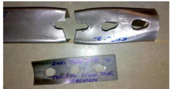
Figure 15: Bearing + rupture failure
