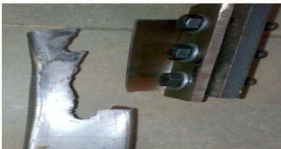
Figure 16: Block shear failure
