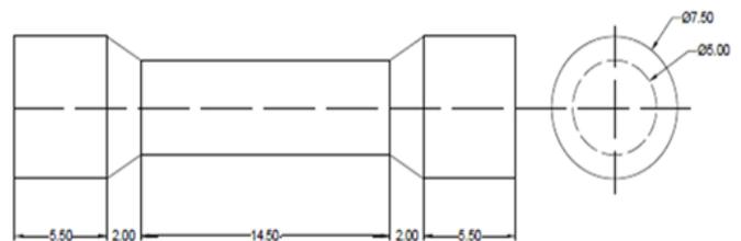
**Figure.3:** Test Specimen geometry
