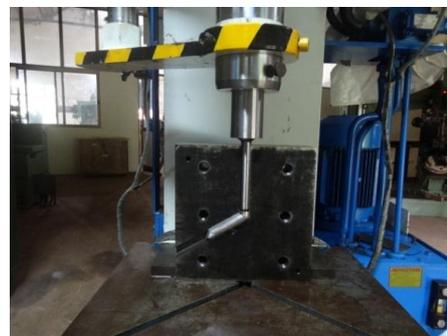
**Figure.1:** Experimental Setup of ECAE process
