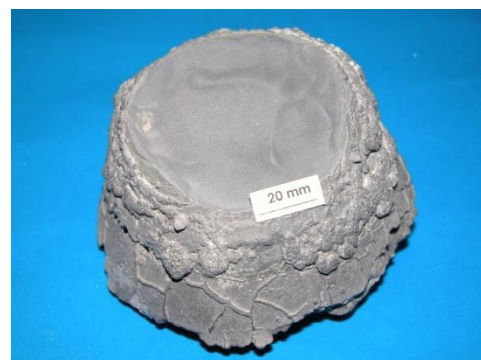
Figure 1: A large specimen of SiC p /Al 2 O 3 composite prepared by directed metal oxidation process in a conical shape. We note that the SiC p /Al 2 O 3 composite thus obtained has the shape of the mould.
