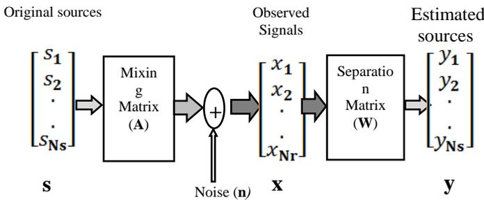
**Figure.1.** BSS schematic diagram
