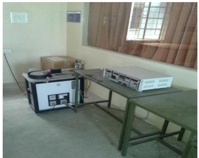
**Figure 1.** Pin on Disc Apparatus
