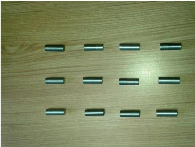
Figure 2. Specimens prepared for wear test
