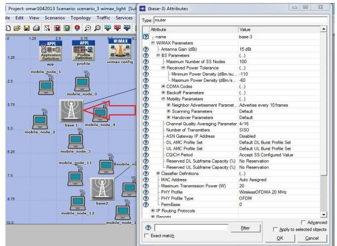
Figure 3: WiMAX bases stations configuration
