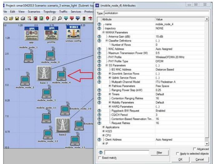
Figure 4: WiMAXs Mobile node configuration
