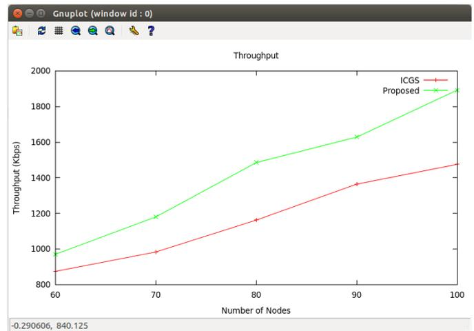
Fig shows the results of throughput with respect to number of nodes in the network. It is already stated that, nodes which have more capability of replenishing their energy will participate in data transmission. And, it is proved from the proposed algorithm that, reliability is directly proportional to expense of energy. Therefore, throughput of the network gives satisfactory results compared to ICGS protocol.
