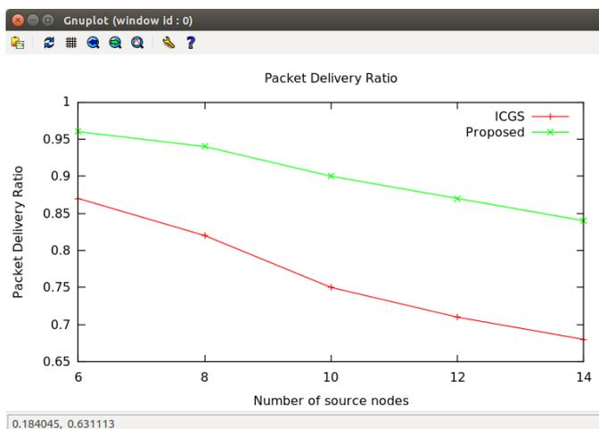
Fig shows the results of packet delivery ration with respect to source nodes. Increase in number of source node lead to allocation of more time slots. But, the tour interval is fixed, then there might be delay in delivering the data. Hence, there
