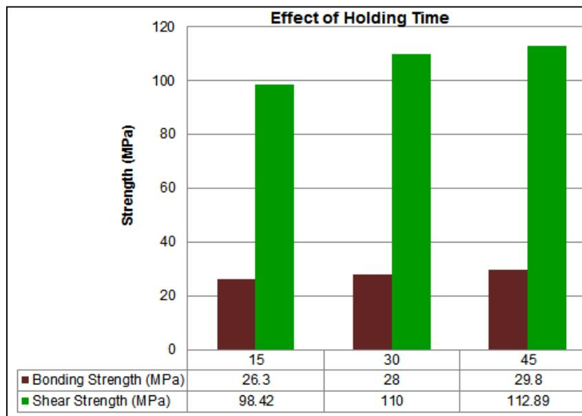
Figure 10. Effect of Holding Time on Bonding and Shear strength
