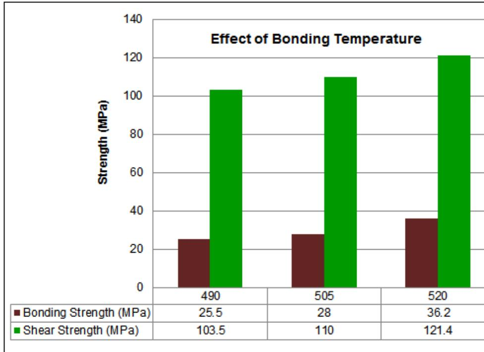
**Figure 6.** Effect of Bonding Temperature on Bonding and Shear strength
