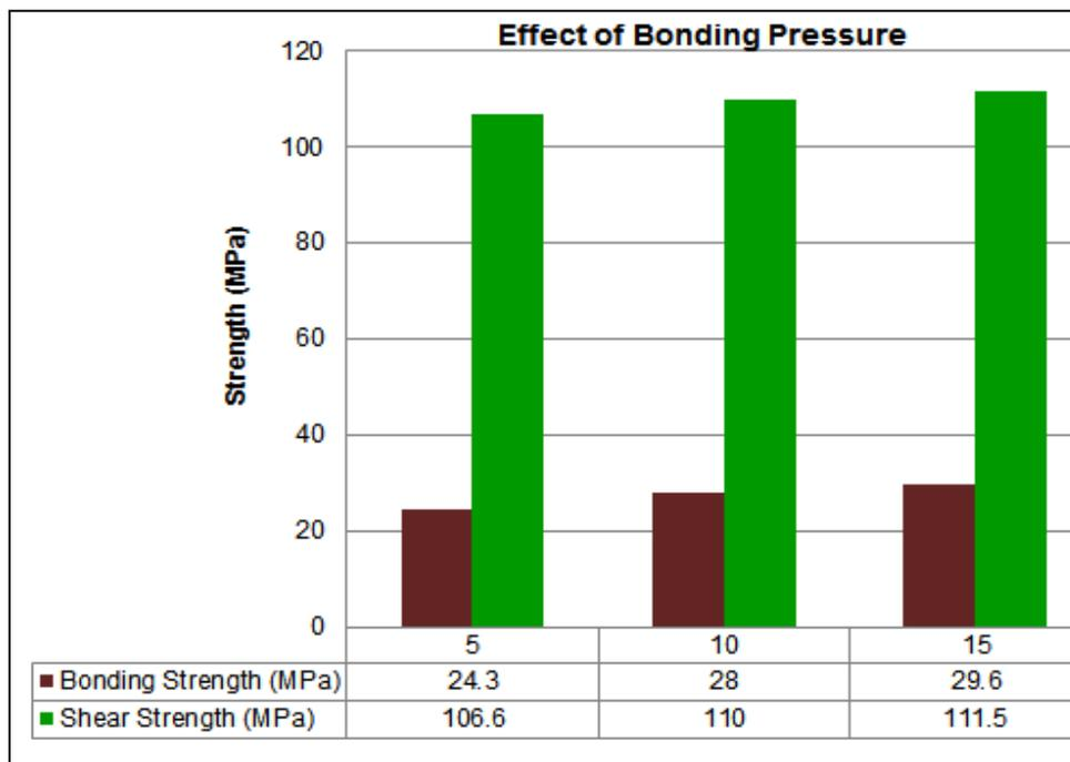
**Figure 8.** Effect of Bonding Pressure on Bonding and Shear strength
