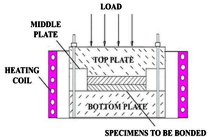
**Figure 2.** Diffusion Bonding Set up
