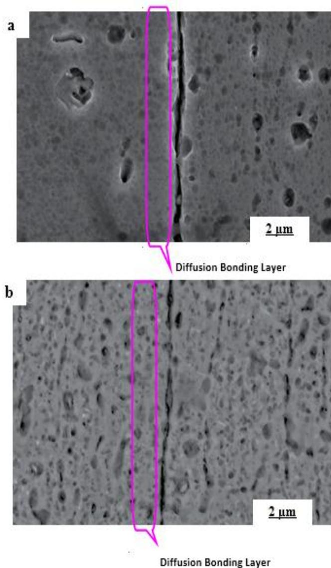
**Figure 12.** SEM images of diffusion bonded AA7075 aluminium alloy joints
