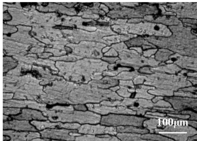
**Figure 1.** Microstructure of AA7075 aluminium alloy
