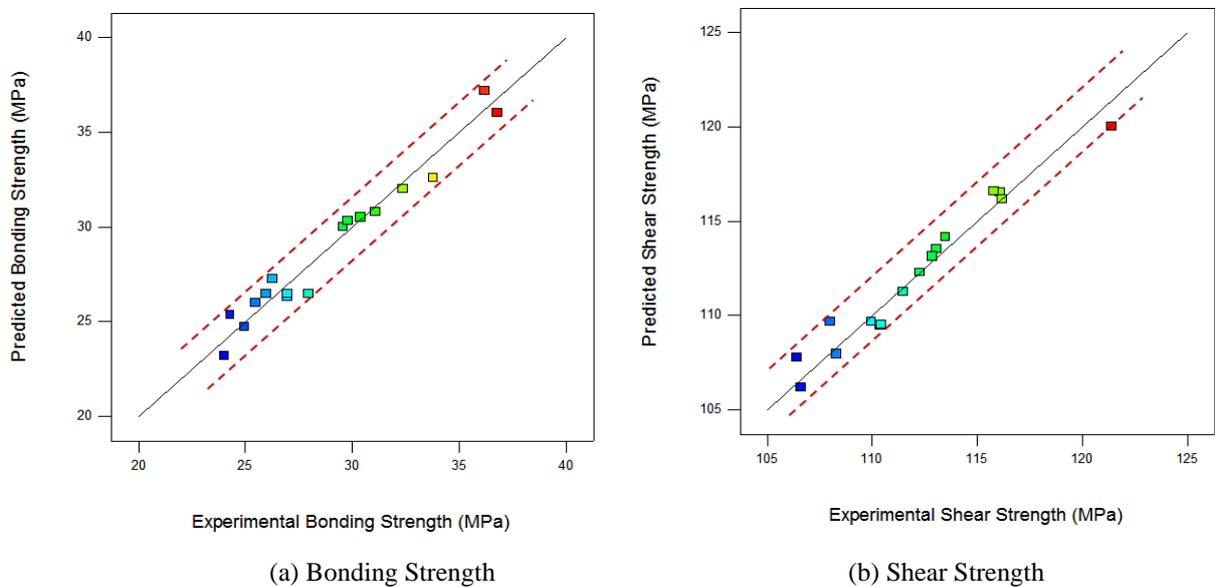
Figure 5. Correlation of the Response (Bonding and Shear Strength)
