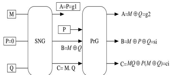
Figure 6. Design of full adder
