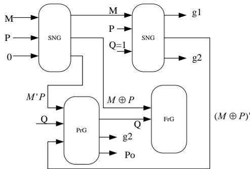
**Figure 7.** Design of full adder
