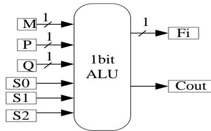
**Figure 8.** Design of 1bit ALU
