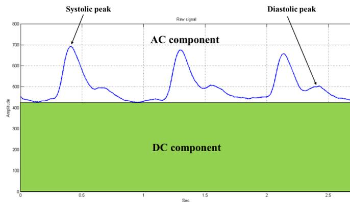
**Figure 1.** PPG signal with AC and DC components
