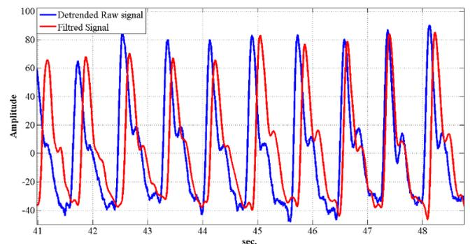
**Figure 4.** Raw and filtered PPG signal
