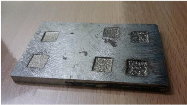
Figure 1. Square hole on Stainless Steel
