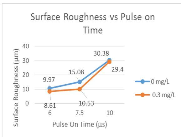
**Figure 7.** Relation of Surface roughness with pulse  $T_{on}$
