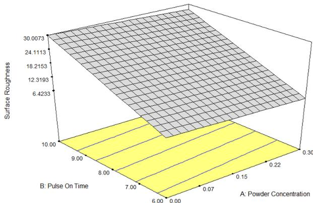
**Figure 5.** Effect of  $T_{on}$  on time and powder concentration on  $R_a$
