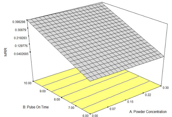
Figure 3. Effect of  $T_{on}$  on time and powder concentration on MRR
