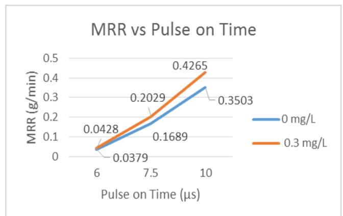
Figure 4. Relation of  $T_{on}$  on MRR
