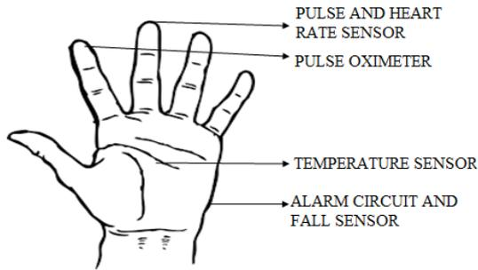
**Figure 3.** Positioning of sensors
