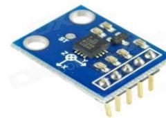
**Figure 6.** GY-61 accelerometer
