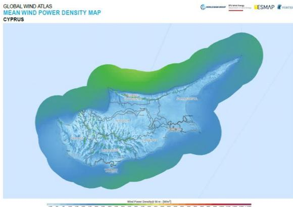
Figure 4. Mean wind power density map at 50m height
