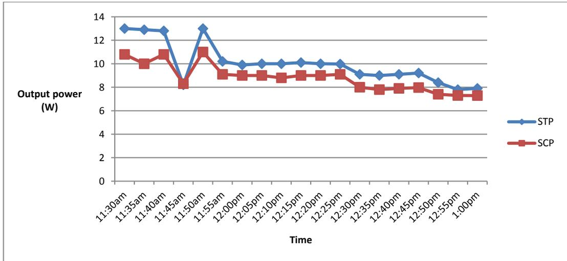
Figure 1.5: Output power variation in solar tree and conventional panel.
