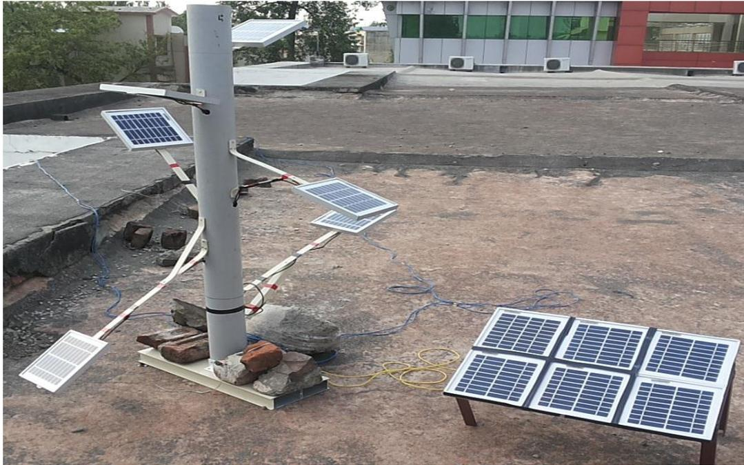
**Figure 1.3:** Experimental Solar-Tree and Fixed Solar Panel
