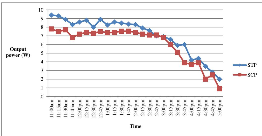
Figure 1.6: Output power variation in solar tree and conventional panel.
