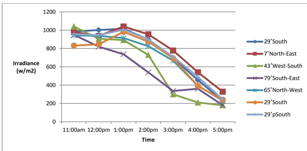
Figure 1.7: Irradiance variation on the different panels of the solar tree.
