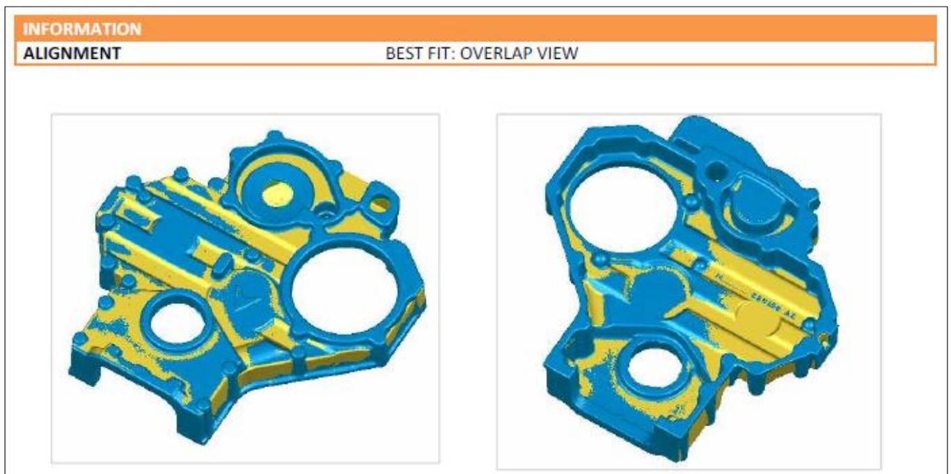
**Fig.4** Overlapping of the scanned model and machining model
