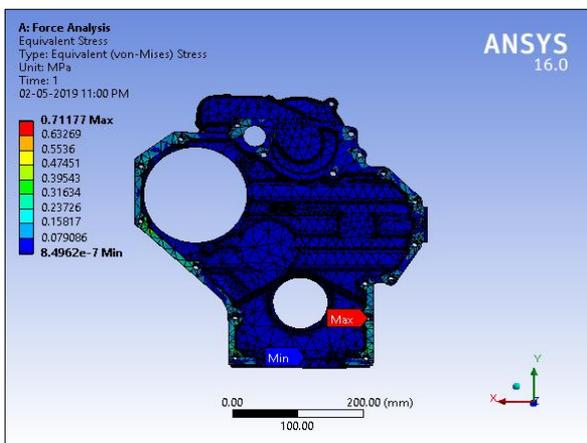
Fig.12 Equivalent stress in force analysis
