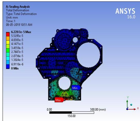
Fig.13 Total deformation for sealing analysis
