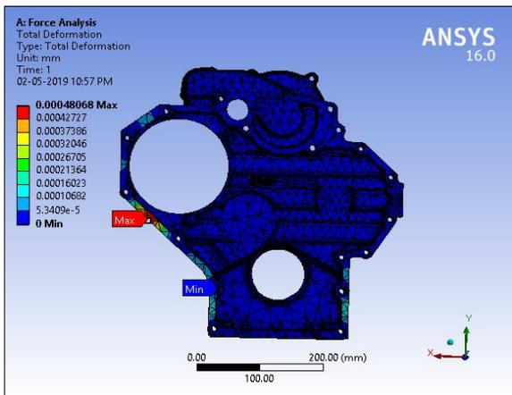
Fig.11 Total deformation in force analysis
