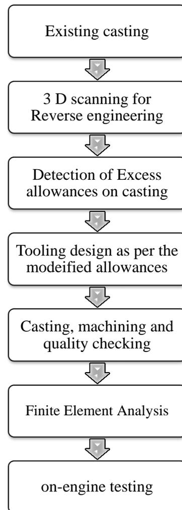
**Fig.1** Flowchart of the methodology for weight optimization of gear casing
