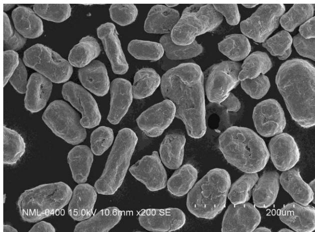
**Fig.1:** SEM micrograph of low carbon content ferrous powders.
