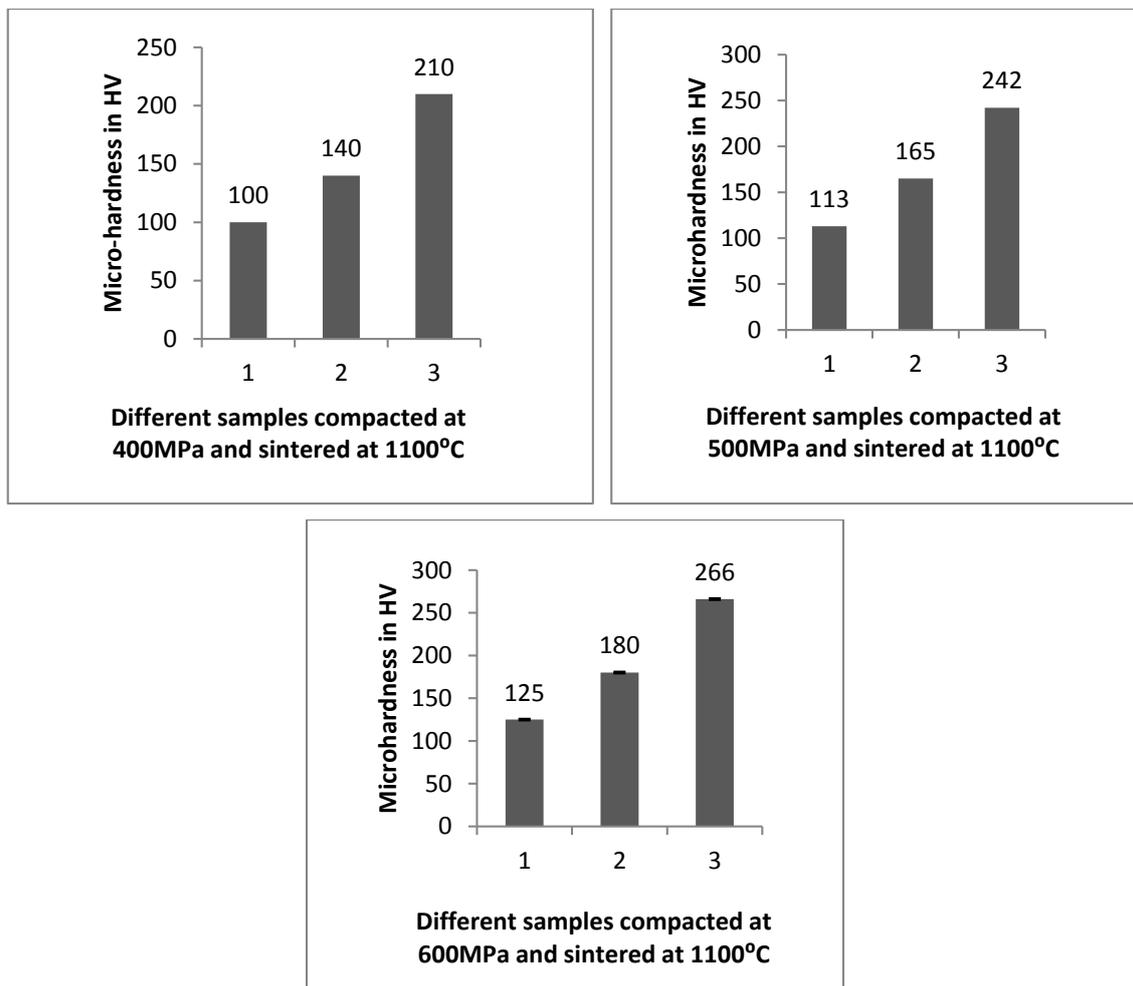
**Fig.2:** Micro-hardness values for different sintered compact samples : (1)LCFP(bal)+2wt% Cu+ 0.2wt%C, (2) LCFP(bal)+2wt% Cu+ 0.5wt%C (3) and LCFP(bal)+2wt% Cu+ 1wt%
