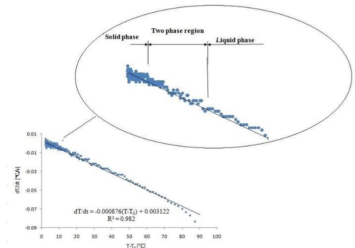
**Figure 7.**  $dT/dt$  versus  $(T-T_0)$  curve of WCOME during cooling
