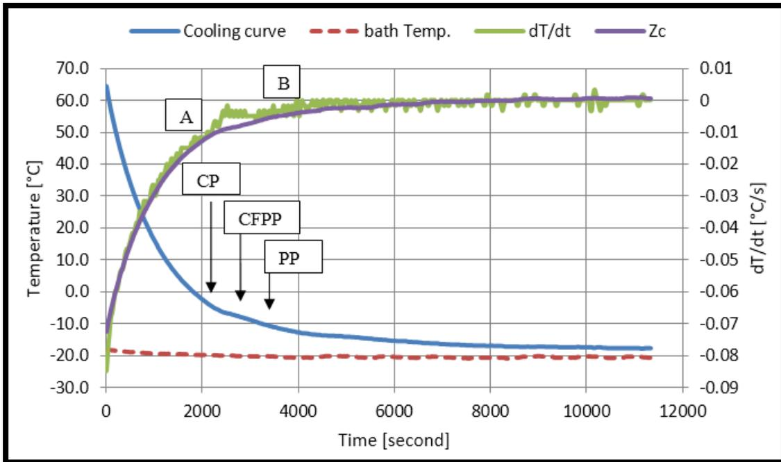
**Figure 8.** Cooling curve analysis and Newtonian zero curve of RCOME
