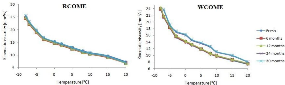
Figure 3. Measured kinematic viscosities of biodiesel samples from  $-10^\circ\text{C}$  to  $20^\circ\text{C}$
