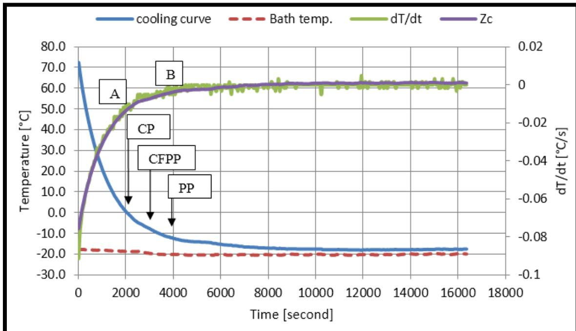
**Figure 9.** Cooling curve analysis and Newtonian zero curve of WCOME
