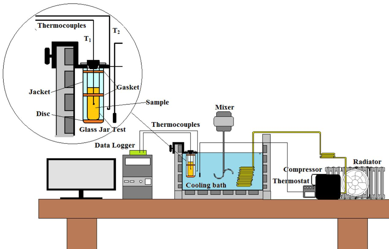
Figure 1. Experimental setup for CA-CCA
