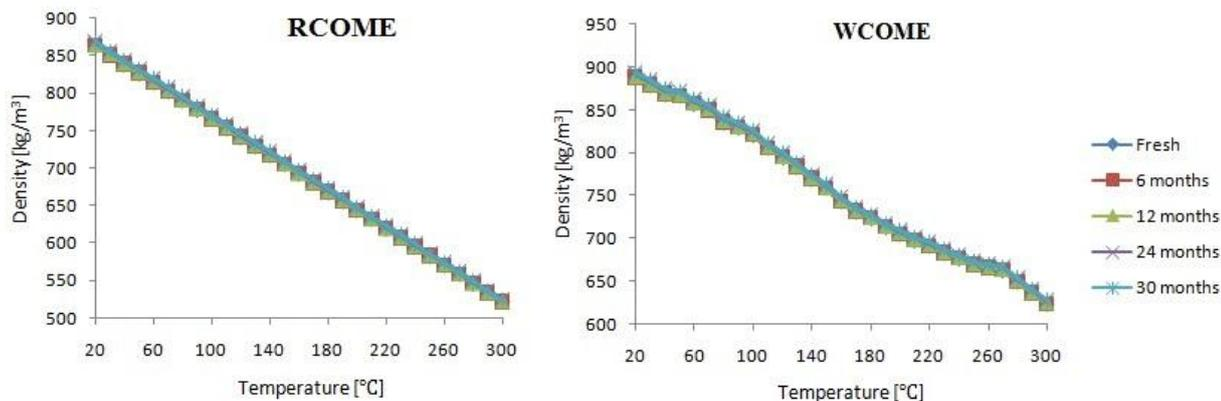
**Figure 4.** Measured Density of biodiesel sample from 20°C to 300°C
