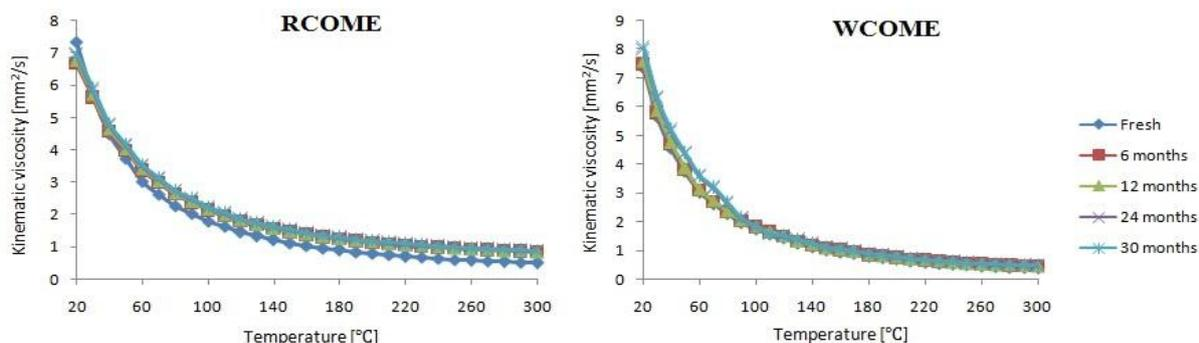
Figure 2. Measured kinematic viscosities of biodiesel samples from  $20^\circ\text{C}$  to  $300^\circ\text{C}$
