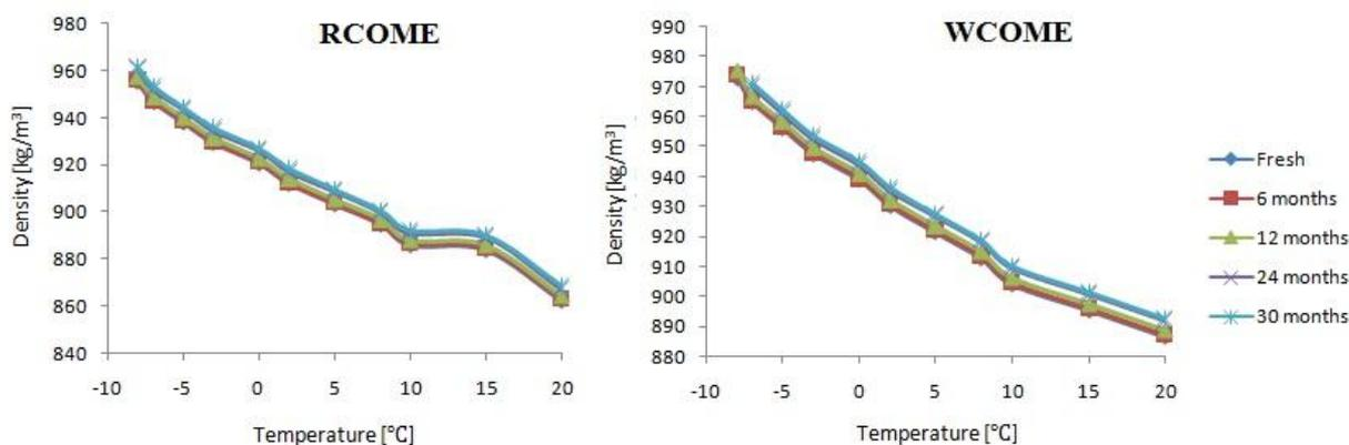
**Figure 5.** Measured Density of biodiesel sample from -10°C to 20°C
