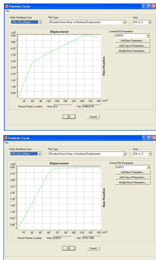
**Figure 2.** Pushover Curves in transverse and longitudinal direction for T girder
