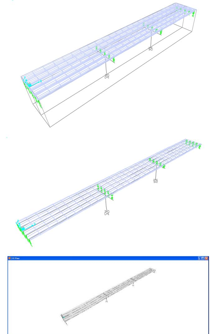
**Figure 1.** Finite element model for T, I and box girders three span bridges
