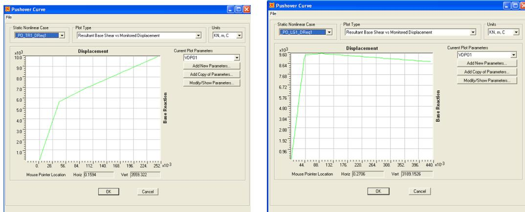
Figure 3. Pushover Curves in transverse and longitudinal direction for I girder
