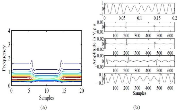
**Fig. 3:** Localization of pure sine wave in (a) S-transform (b) SGWT decomposition
