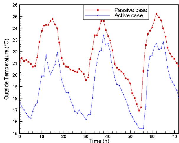
**Fig.4.** Outside temperature variation, passive and active cases.
