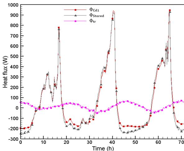
**Fig.15.** Heat fluxes, transmitted through the wall 2, stored in PCM and transmitted to the cavity, case of active study.
