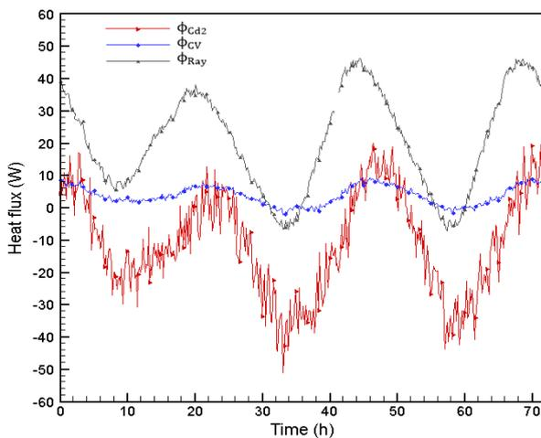
**Fig.14.** Heat fluxes transmitted from PCM to the air layer, case of active study
