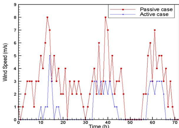
Fig.5. Wind speed variation, passive and active cases.
