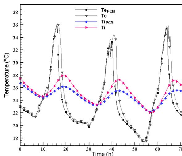
Fig.7. Temperature variation on internal and external faces of the western walls with and without PCM, September 14th to 16th, 2016.
