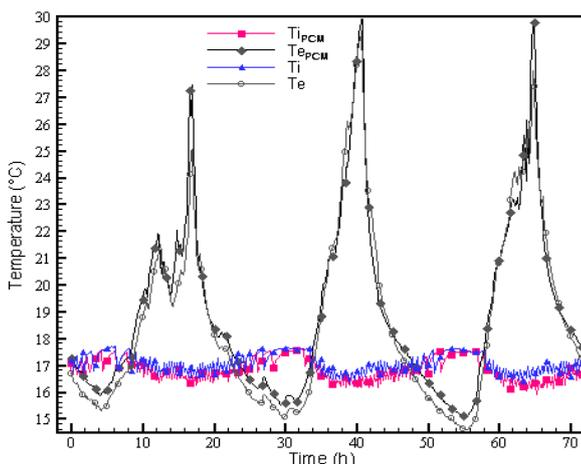
**Fig.9.** Temperature Variations of the inside and outside faces of the western walls with and without PCM, October 14<sup>th</sup> to 16<sup>th</sup>, 2016.
