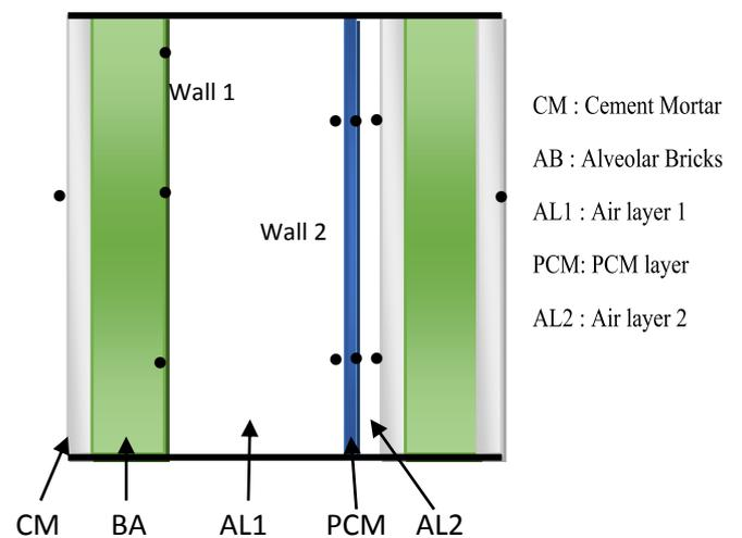
Fig.2. Western walls composition and thermocouples positions
