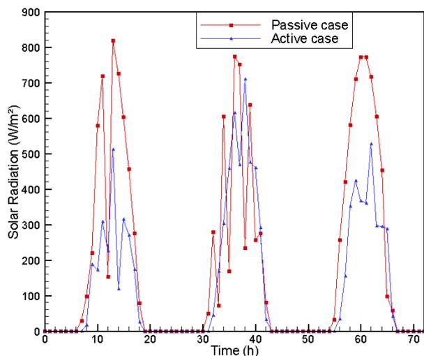
Fig.6. Solar radiation variation, passive and active cases.
