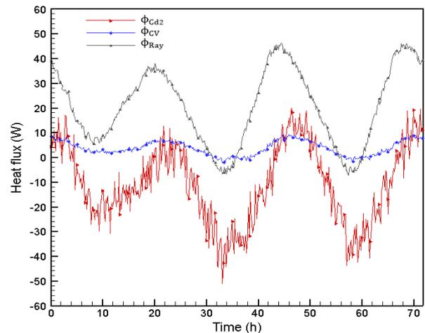
Fig.12. Heat fluxes transmitted from PCM to the air layer, passive study
