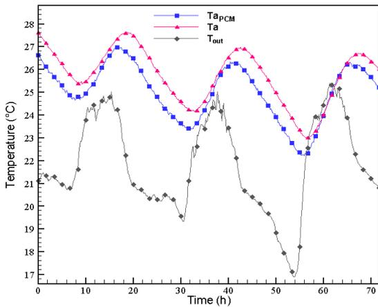
**Fig.8.** Variations of the ambient temperatures of the cavities with and without PCM, September 14th to 16th, 2016.
