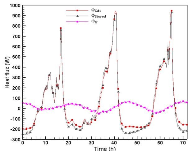
Fig 13. Heat fluxes, transmitted through the wall 2, stored in PCM and transmitted to the cavity, passive study.
