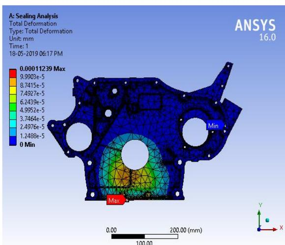
**Fig. 17** Total deformation for sealing analysis
