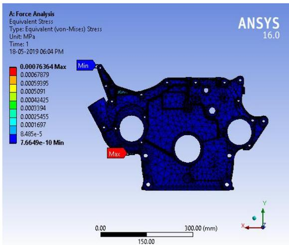
**Fig. 16** Equivalent stress of front cover
