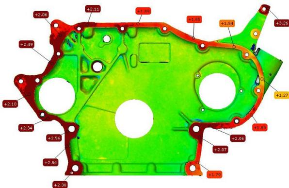
**Fig. 4** Geomagic analysis of mounting side
