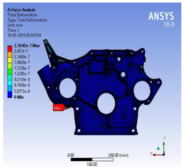
**Fig. 15** Total deformation of front cover
