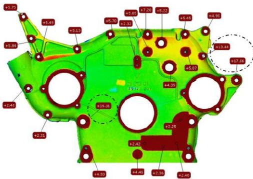
**Fig. 3** Geomagic analysis of outer side
