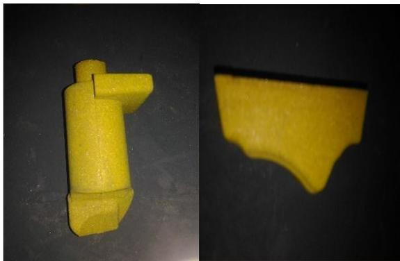
**Fig. 8** Sand cores
