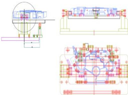
**Fig. 13** Index able VMC holding fixture
