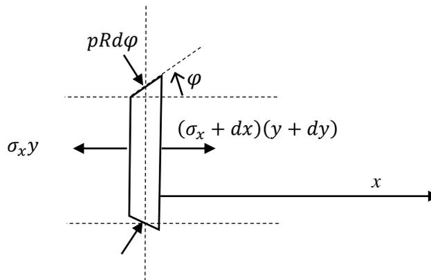
Figure. 2. An element of strip and the stresses acting on it
