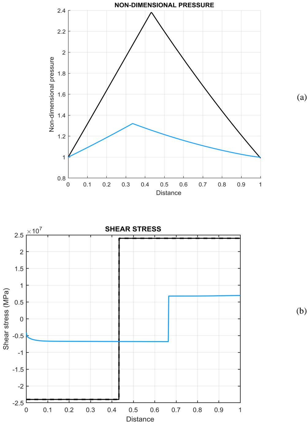
Figure 6. Comparison between the full-film and mixed-film lubrication for (a) pressure and (b) shear stress
