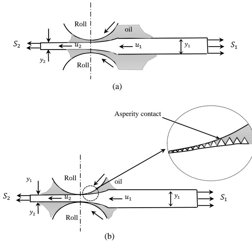
Figure .1. (a) strip rolling in full-film regime and (b) mixed-film lubrication
