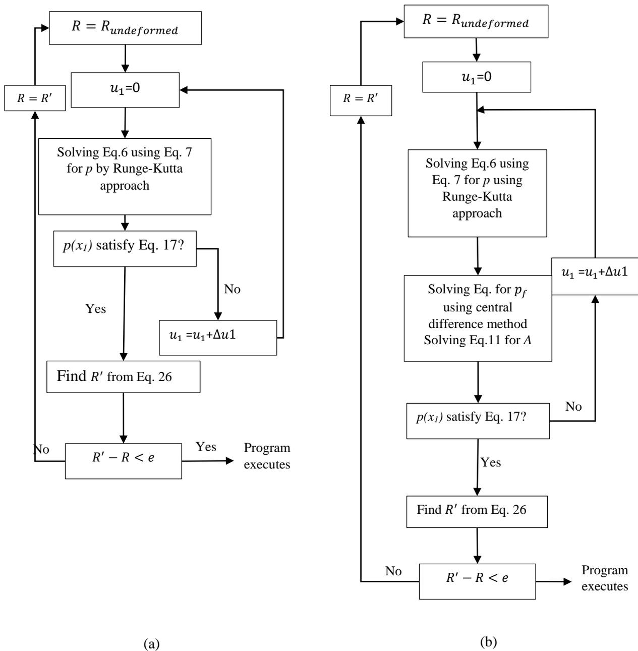
**Figure 5.** Numerical procedure flow chart for (a) full-film regime and (b) mixed-film regime.
