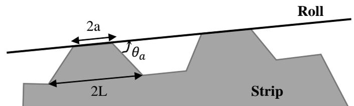
Figure 3. Schematic of asperity in contact with roll
