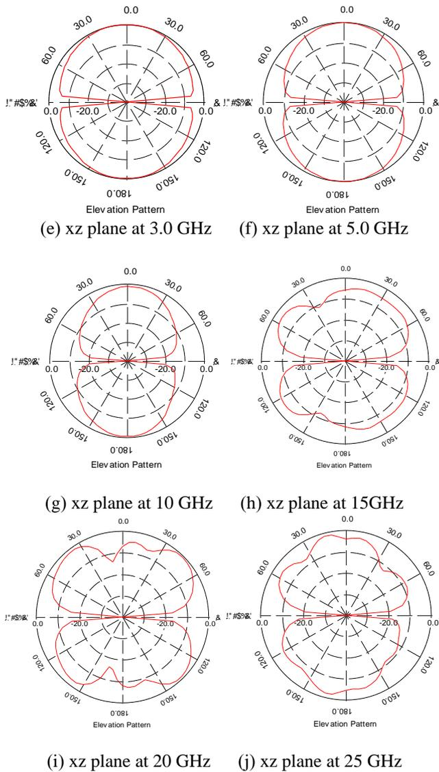
**Figure 12.** Radiation pattern of proposed slot antenna
