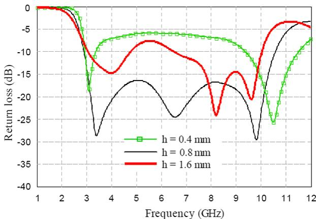
**Figure 8:** The return loss ( $S_{11}$ ) of the slot antenna in the case adjusting h
