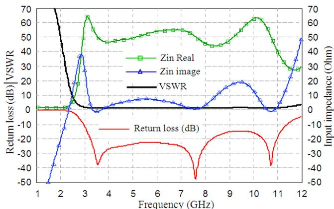
**Figure 9:** The return loss ( $S_{11}$ ) of slot antenna with SRR tuning stub
