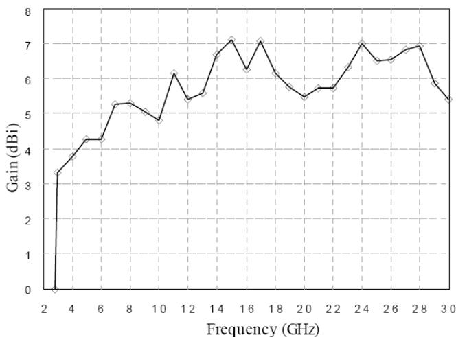
**Figure 13:** Gain of proposed slot antenna
