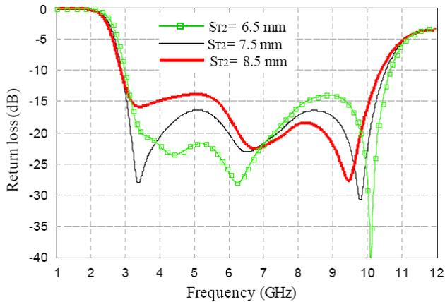
**Figure 4:** The return loss ( $S_{11}$ ) of the slot antenna in the case adjusting ST2.
