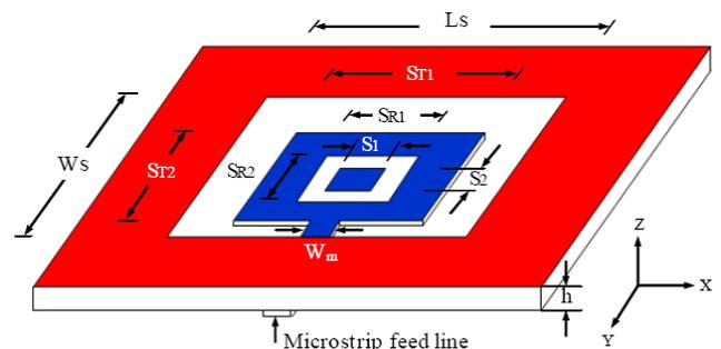
**Figure 1:** Structure of slot antenna using microstrip feed line with slot-ring resonator in rectangular tuning stub
