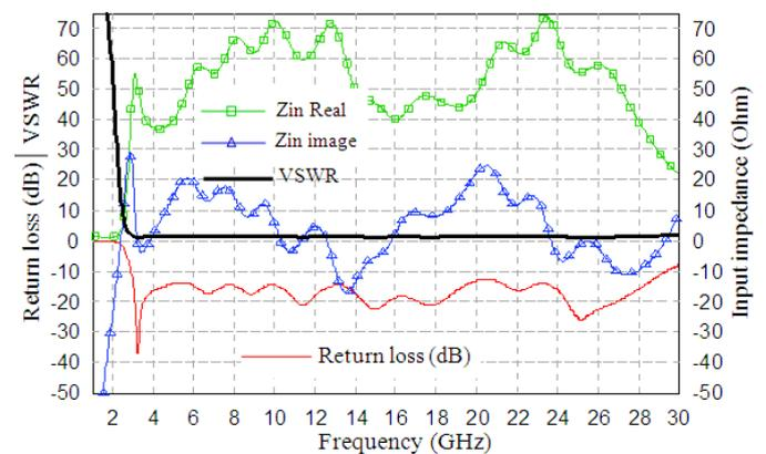
**Figure 10:** The return loss ( $S_{11}$ ) of the slot antenna in the case shifted left/right of SRR in tuning stub
