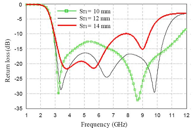
**Figure 3:** The return loss ( $S_{11}$ ) of the slot antenna in the case adjusting ST1.
