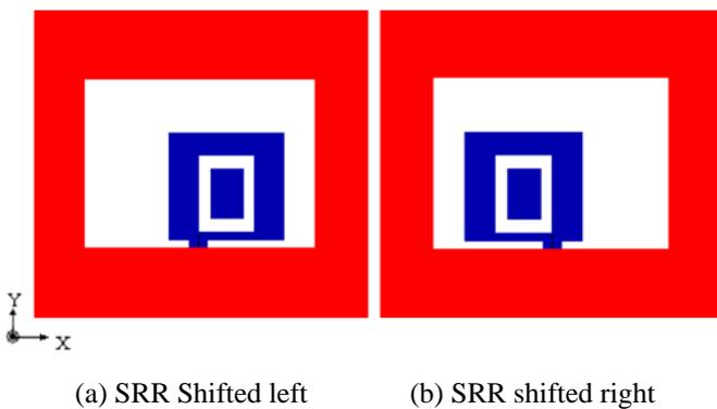
**Figure 2:** slot antenna using microstrip feed line with slot-ring resonator with tuning stub in case shift left and right of tuning stub
