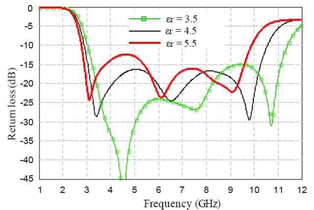
**Figure 7:** The return loss ( $S_{11}$ ) of the slot antenna in the case adjusting dielectric constant ( $\epsilon_r$ )
