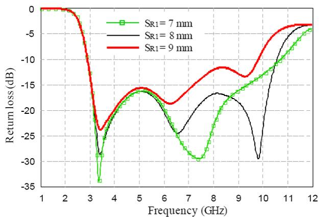
**Figure 5:** The return loss ( $S_{11}$ ) of the slot antenna in the case adjusting SR1.
