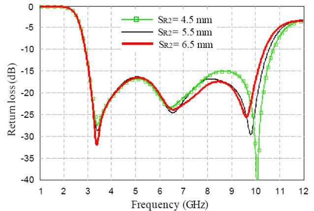
**Figure 6:** The return loss ( $S_{11}$ ) of the slot antenna in the case adjusting SR2.
