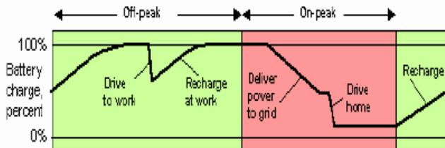
Figure 6. Representation of charging and discharging of battery by EV user
