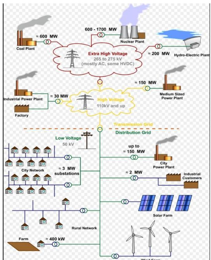
Figure 1. Representation of Grid Technology
