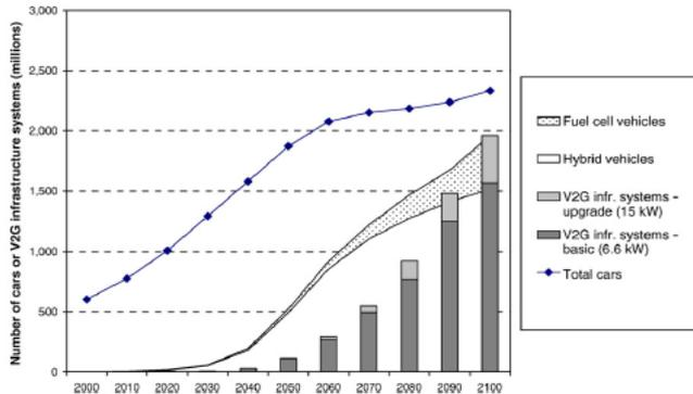
Figure 5. Global deployment of V2G technology
