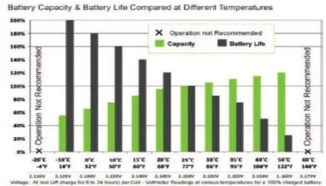
Figure 7. Charging and discharging capacity of Battery
