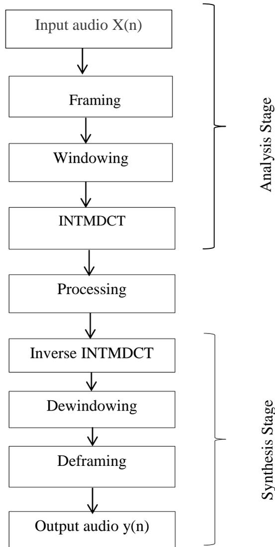
**Fig.1 Block diagram of proposed method**
