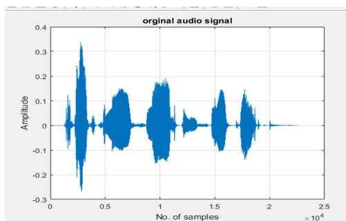
**Fig.2.** Input Audio Signal with the sampling rate of 44.1 KHz which is in .Wav format
