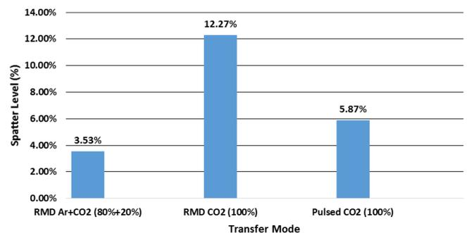
**Fig 14.** Spattering Percentage Comparison Chart
