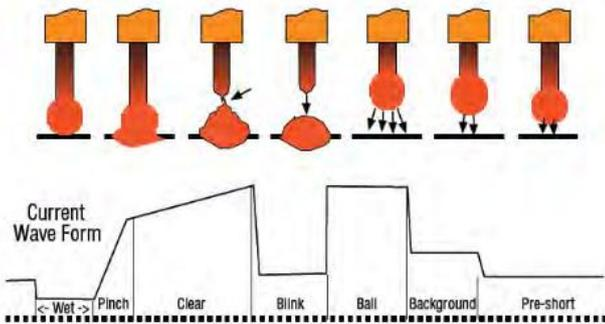
Fig 3. Work principle of RMD
