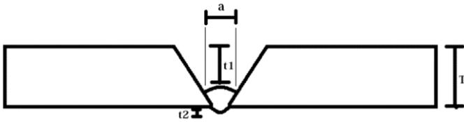
**Fig 9.** Weld deposition calculation
