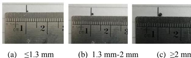
**Fig 8.** Classify of spatter diameter
