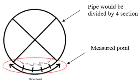
**Fig 7.** Root reinforcement measured point
