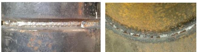
(a) Root pass outer 2R position (b) Root pass penetration 2R position
