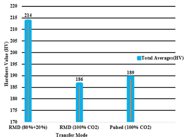
**Fig 15.** Hardness value chart on weld metal
