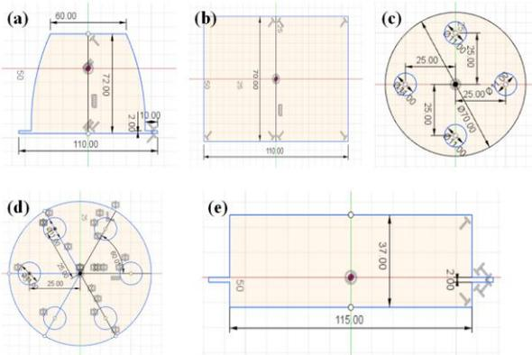
**Figure 2:** CAD design of pellet mixer parts (a) bottom case, (b) top case, (c) sample holder-1, (d) sample holder-2 and (e) top case cap.
