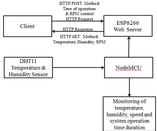
**Figure 7:** Block diagram of embedded system.
