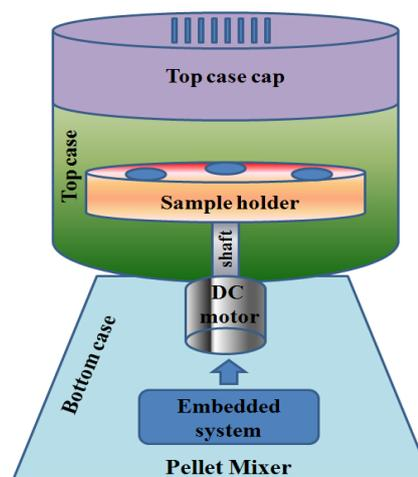
Figure 1: Block diagram of Pellet mixer.
