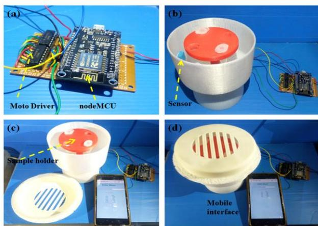
**Figure 9:** Mobile interfaced pellet mixer (a) control circuit. (b) sensor attachment, (c) sample attachment and (d) mobile interface system.
