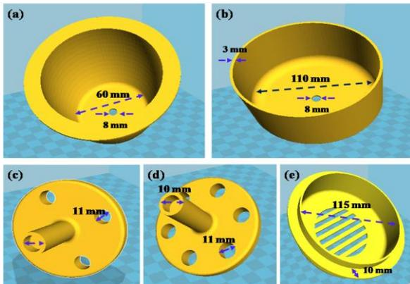
**Figure 3:** STL files of pellet mixer parts (a) bottom case, (b) top case, (c) sample holder-1(d) sample holder-2 (e) top case cap.
