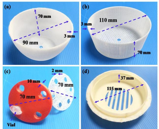
**Figure 5:** 3D printed files of pellet mixer parts (a) bottom case, (b) top case, (c) sample holders and (d) top case cap.
