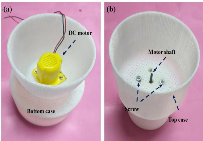
**Figure 6:** Assembly of motor.
