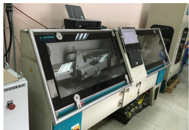
Fig.4. Hamburg means of rut formation estimation HWTD
