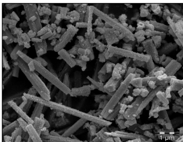
**Figure 2:** SEM micrograph of the synthesized polyrhodanine tubes coated with silver nanoparticles (reaction time=24 h)
