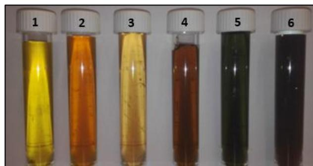
**Figure 3:** Varied reaction times for silver nanoparticle formation. (1) t=0, (2) t=1.5, (3) t=3, (4) t=8, (5) t=12, and (6) t=24 hours
