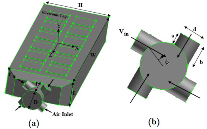
**Fig. 1.** Schematic of the geometry of the printed circuit board assembly used in this study (a). The printed circuit board channel equipped with 12 electronic chips (30 x 15 x 3 mm/chip) with a total heat generation of 24 W (2 W/chip) (b). Vortex generator that shows the generation of vortices inside the PCB channel.
