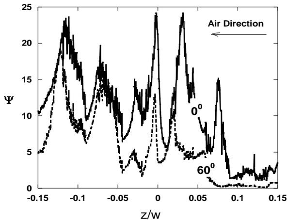
**Fig.4 :** Dimensionless temperature at the upper surface
