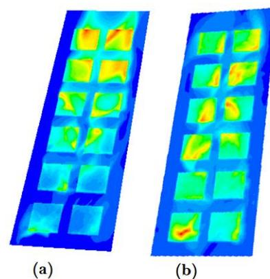
Fig. 2: Contour of static temperature at the upper surface: (a)  $\phi = 0^\circ$ , (b)  $\phi = 60^\circ$
