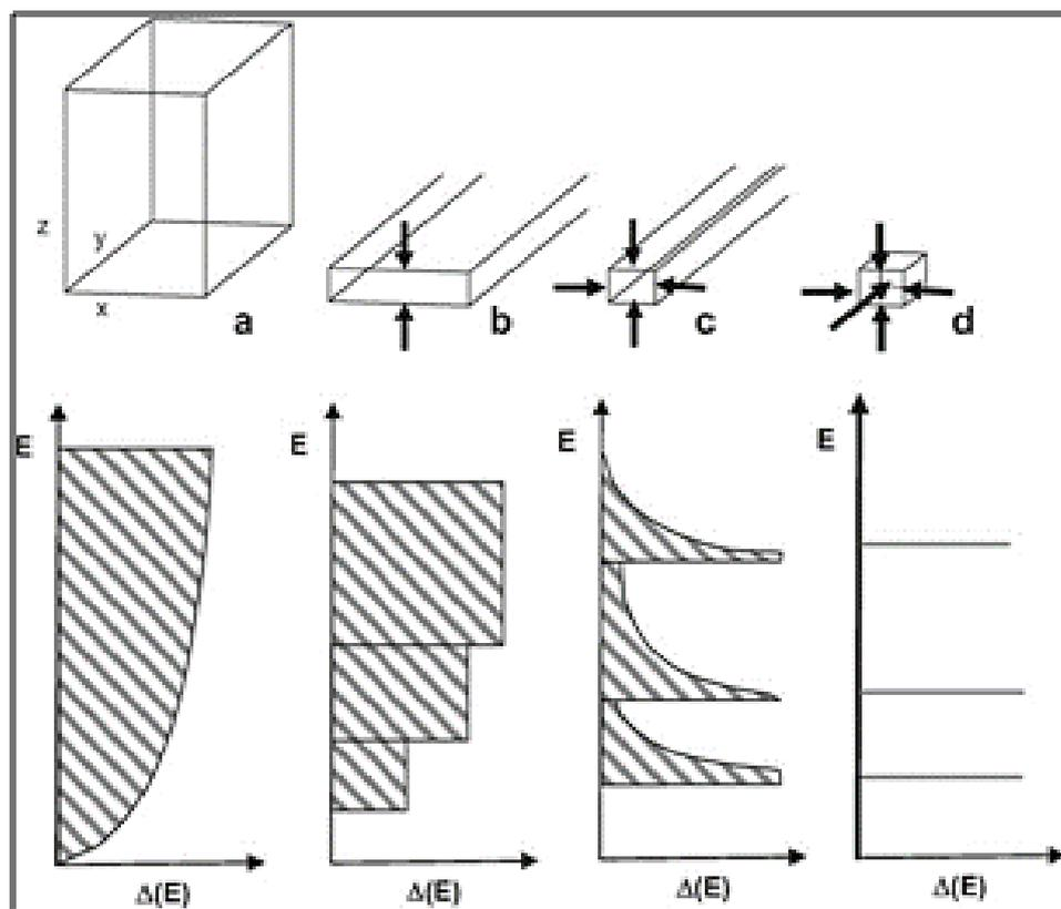
**Figure 1.** Schematic drawing to show the concept of system dimensionality: (a) bulk semiconductors (3D); (b) thin film, layer structure, quantum well (2D); (c) linear chain structure, quantum wire (1D); (d) cluster, colloid, nanocrystal, quantum dot (0D). In the bottom, the corresponding density of states  $\Delta(E)$  versus energy (E) diagram (for ideal cases)
