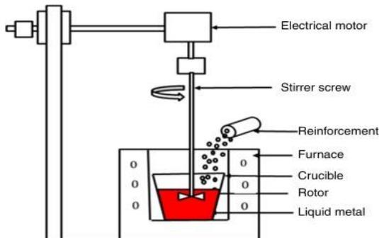
Figure 1: Stir casting Investigational set up (Maruyama [17])
