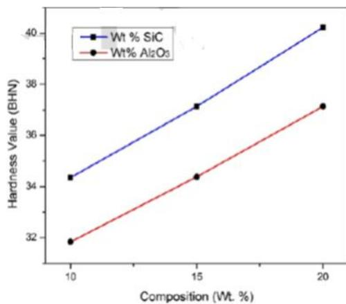
**Figure 5:** Showing the variation of hardness value with composition of Al<sub>2</sub>O<sub>3</sub> and SiC (Ashwath et al [21])
