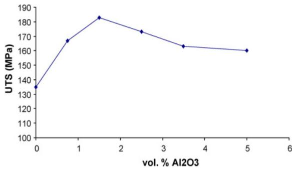
**Fig: 4** Variation of UTS with Al<sub>2</sub>O<sub>3</sub> content (Mazahery et al [20])
