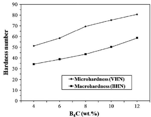
Fig: 2 Variety of hardness with B<sub>4</sub>C content (Kakaiselvan et al [18])
