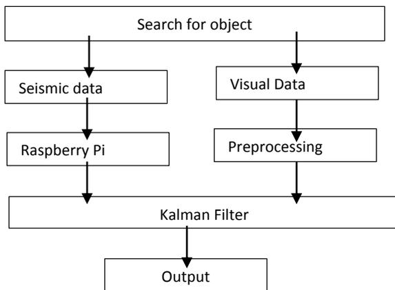
1. Capture Image and Seismic data : this is done by using ADXL335 with Raspberry pi board with webcam.
