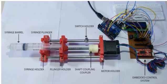
**Figure 3:** 3D printed infusion pump
