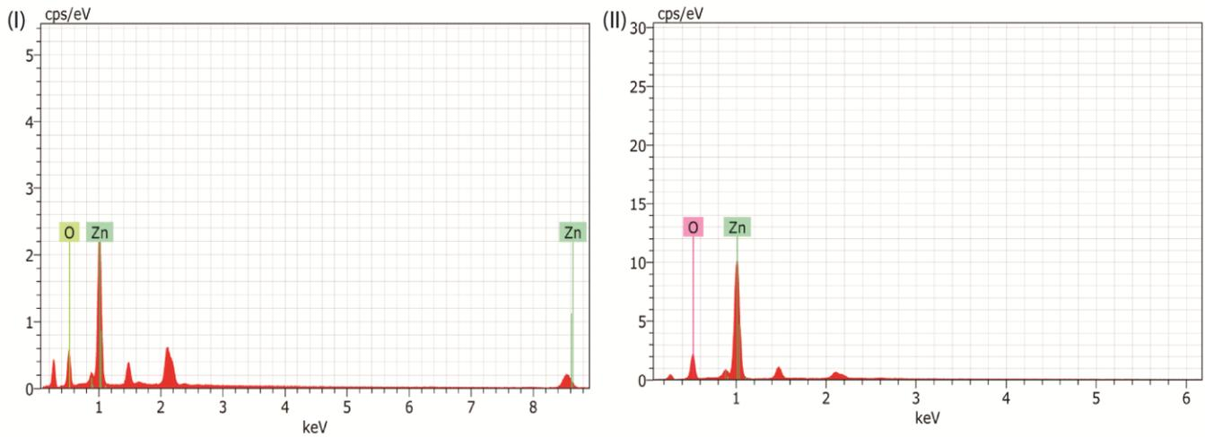
**Figure 8:** Elemental analysis by EDS of ZnO nanomaterials synthesized using (I) Burette setup and (II) 3D printed infusion pump
