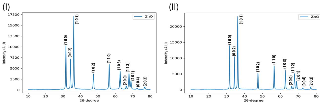
**Figure 6: XRD of ZnO nanomaterials synthesized using (I) Burette setup and (II) Infusion pump**
