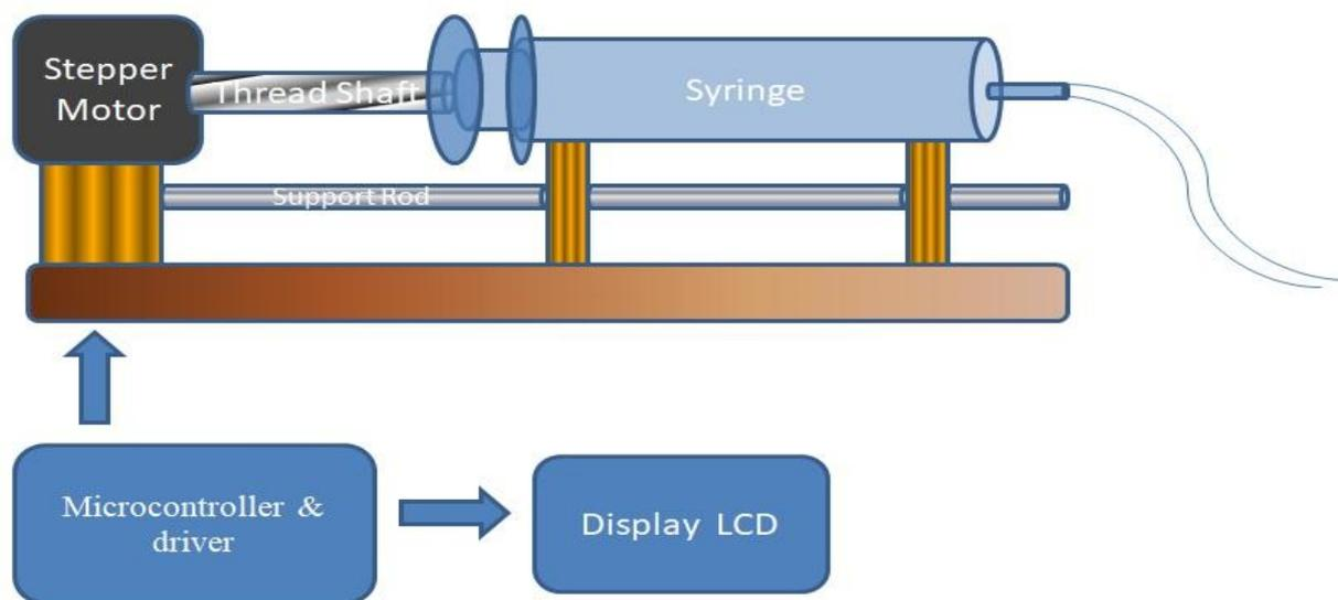
**Figure 1: Schematic representation of the infusion pump**
