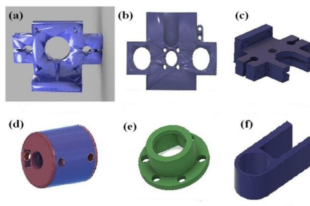
**Figure 2: 3D printed infusion pump parts** (a) Motor holder, (b) Syringe plunger holder, (c) syringe holder, (d) shaft coupling coupler, (e) shaft connector coupling and (f) switch holder
