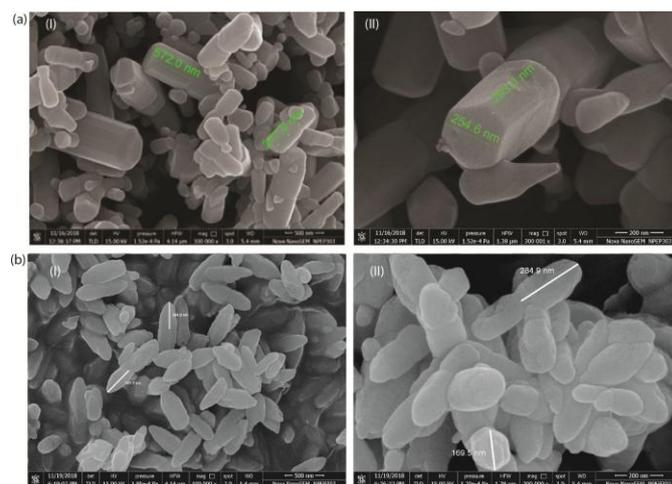
**Figure 7: FESEM images of ZnO nanomaterials synthesized by using (a) 3D printed infusion pump; (I) lower and (II) higher magnification images of pencil like hexagonal ZnO nanorods found to have size in the range of 250 – 295 nm with uniform shape and size distribution. (b) Burette setup; (I) lower and (II) higher magnification images of spindle shaped ZnO nanostructures found to have size in the range of 165 – 290 nm with different size and shapes.**
